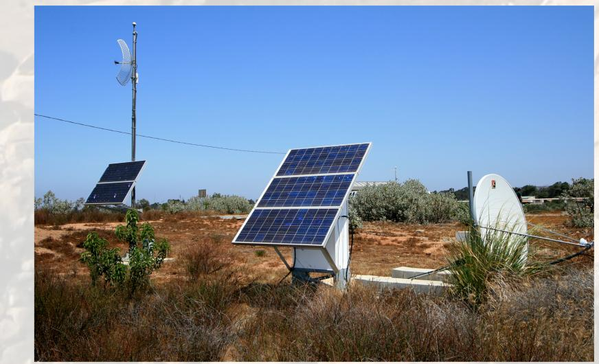
Field-deployed seismic sensors
